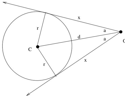
Figure 13.3. Constructing the line tangent to a circle through  $O$ .
