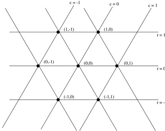
Figure 12.1. A row-column coordinate-system for triangular grids.
