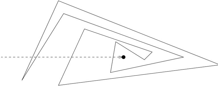
Figure 14.3. The odd/even parity of the number of boundary crossings determines whether a given point is inside or outside a given polygon.
