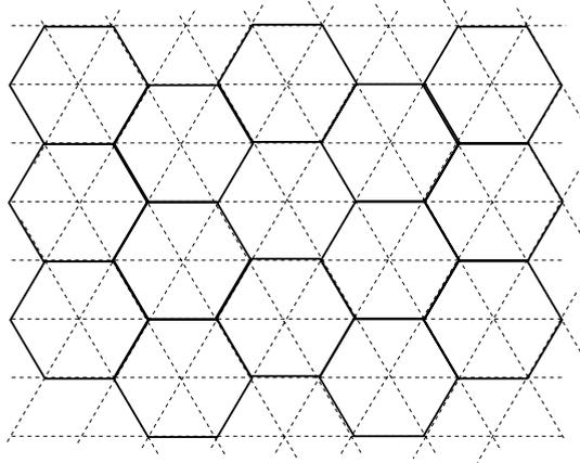
Figure 12.2. Deleting alternate vertices from a triangular lattice yields a hexagonal lattice.
